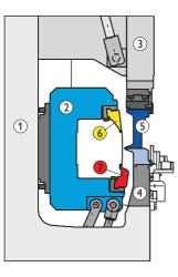
Two frames: the stationary main frame ① of the machine and a C-frame ② with hydraulically actuated swinging movement up-wards or downwards.
