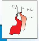
A fundamental characteristic of the EB bending technology is the movement of the blade. The contact line of the blade and the material being bent remains constant. This is achieved by numerically controlled interpolation of the two axes that operate blade movement.
